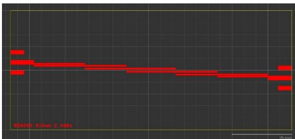
Figure 1: CAD-design of 2.4 GHz bandpass filter for basic material Rogers RO4003C
