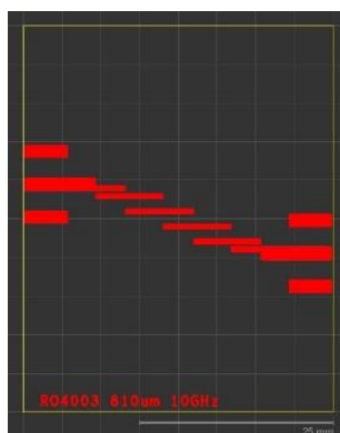
Figure 1: CAD-design of 2.4 GHz bandpass filter for basic material Rogers RO4003C
