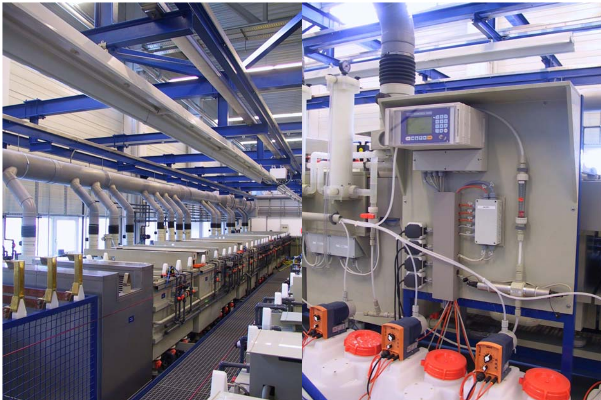
Figure 7: Fully automated plating line with online-analysis (I&T GmbH)
